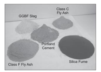
cementitious properties by itself but these are enhanced when it is used with portland cement. Slag is used at 20% to 70% by mass of the cementitious materials.
