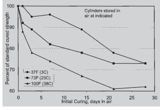
Effect of Non-Standard Curing on Compressive Strength (Ref 5)
