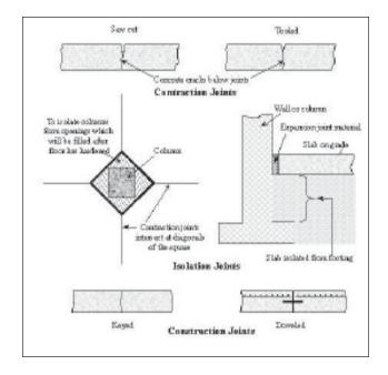
natural tendency to shrink is restrained, tensile stresses that exceed its tensile strength can develop, resulting in cracking.
