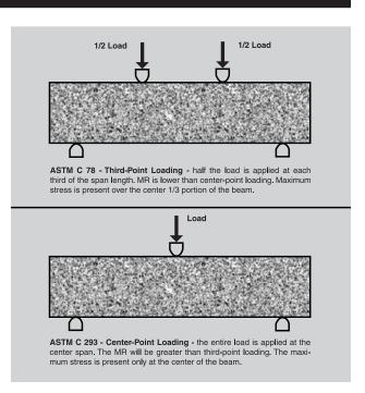
consolidate. *Never allow the beam surfaces to dry at any time*. Immerse in saturated limewater for at least 20 hours before testing.
